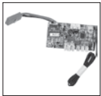
#25 PCP board with ON/OFF switch
